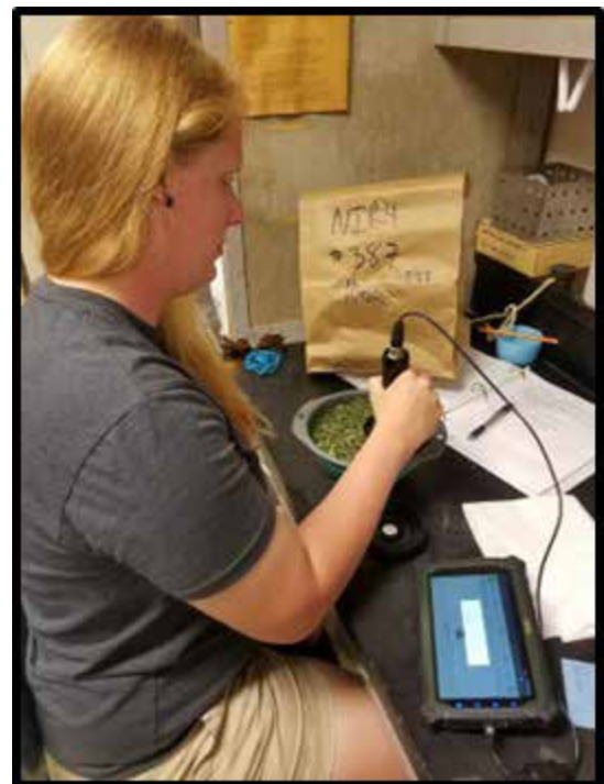
Figure 2. Scanning a dried alfalfa samples using the NIR4 Farm hand-held NIR unit. Photo credit: Liz Patton, UMN.
